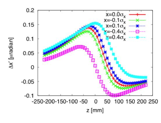
Deflection as function of offset in proton bunch for a beam-beam offset of  $1\sigma_x$
