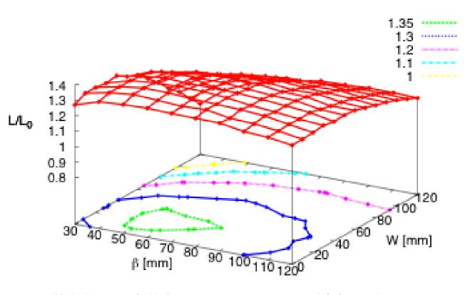
Small gain in LHeC, since only electron beam is disrupted
