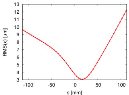
Minimum electron beam size less than half the nominal
