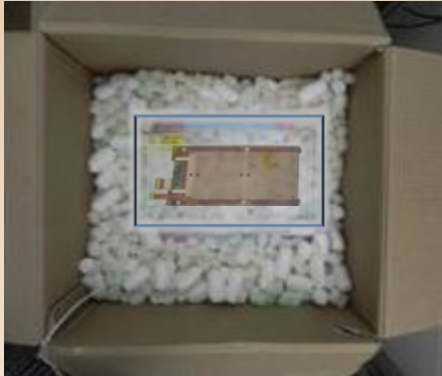
#1) Module on transport plate in plastic box placed inside cardboard box filled with foam chips.
