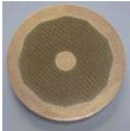
Nb–Ti Strand 1 developed by VNIINM (1.6:1)
