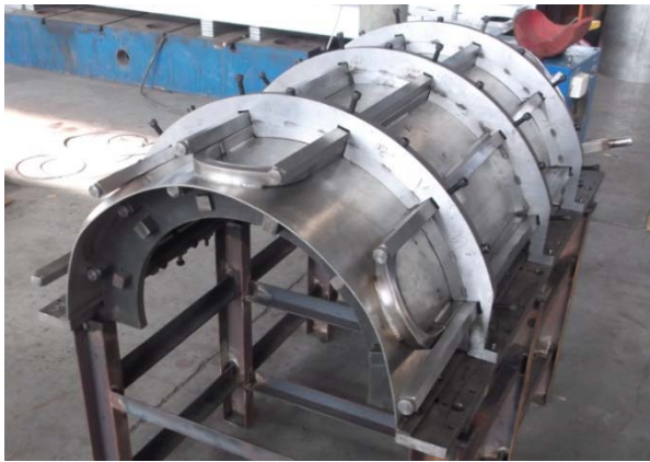
Positioning jig for the welding of thermal shield
