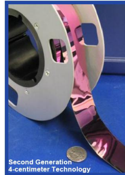
Tape thickness: 0.21- 0.23 mm
