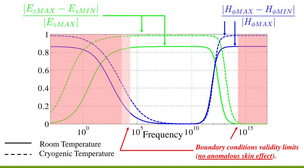
Surface currents are constant over the azimuth (at all the relevant frequencies). The losses in the welding is 5 % of the ones in the copper at room temperature (50% at cryogenic temperatures).
