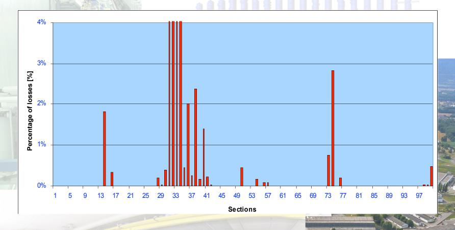
Simulations are consistent: moving the quadrupole in SS05 should set losses to zero in that zone and move them entirely in SS73-77
