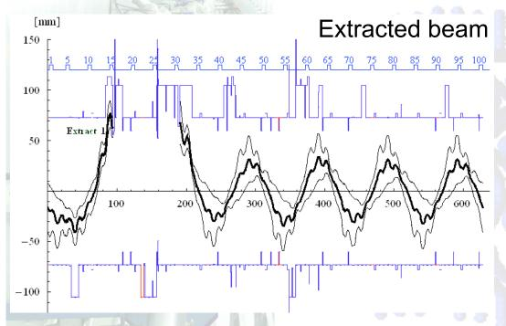
Mechanism generating the loss: particles interacting with the ~ 200 μm thick Mb septum blade are then defocused by the quadrupole in SS5.
