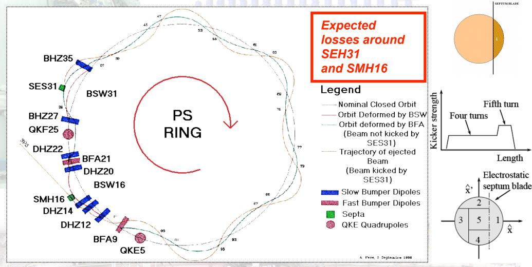
Bump31 (BSW31) to send the beam near the septum 31, about 2 m long BFA9-BFA21 fast kickers (5 turns) to send the beam above the septum 31 Septum31 (SEH31) to slice the beam during the 5 turns QKE16(5-25) to increase the beta and reduce the dispersion to zero at the SEH31 Bump16 (BSW16) to send the beam to SPS Septum16 (SMH16) extraction septum
