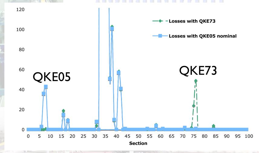
Losses simulated only with slow bumps plus the QKE effect Simulated losses move with the position of the QKE
