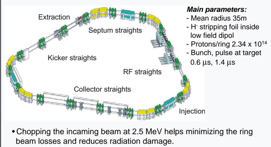
Transverse & longitudinal profiles of injected H<sup>-</sup> beam are cleaned by stripping foils in large 180 ° achromatic bending section.
