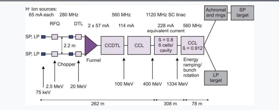
Short description: 2 x 65 mA H<sup>-</sup> beams are combined together at 20 MeV in a funnel section. High frequency Superconducting (SC) cavities accelerate the beam from 400 MeV on. Moderate gradient of 10 MV/m in SC linac is used to keep RF power couplers within reasonable limits. After reducing energy spread by bunch rotation (BR) to ± 2 MeV, halo scraping in large 180 ° achromatic section.
