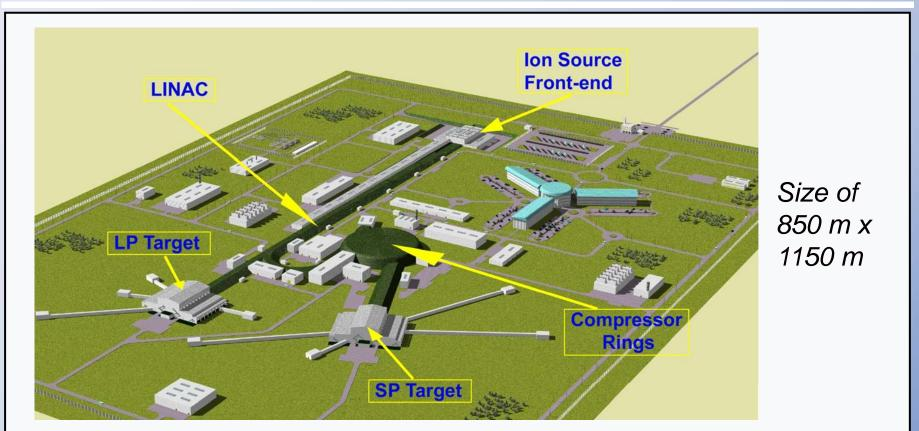
ESS facility consists of a 10 MW, H<sup>-</sup> accelerator capable of delivering 5 MW, 1.4  $\mu$ s pulses to a short pulse (SP) target at 50 Hz & 5 MW, 2 ms pulses to a long pulse (LP) target at 16 2/3 Hz. Both targets have 22 beamlines & liquid Hg is choosen as material.
