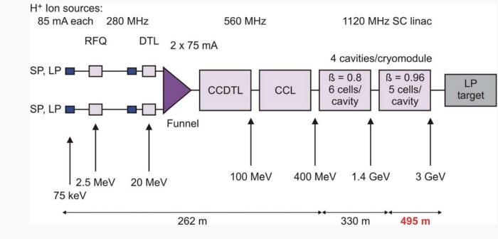
No chopper line & no achromatic bending section. Only 4 % RF d.c. 1 GeV, 5 MW H<sup>+</sup> linac requires only 28 SC cyromodules, 201 m in length.
