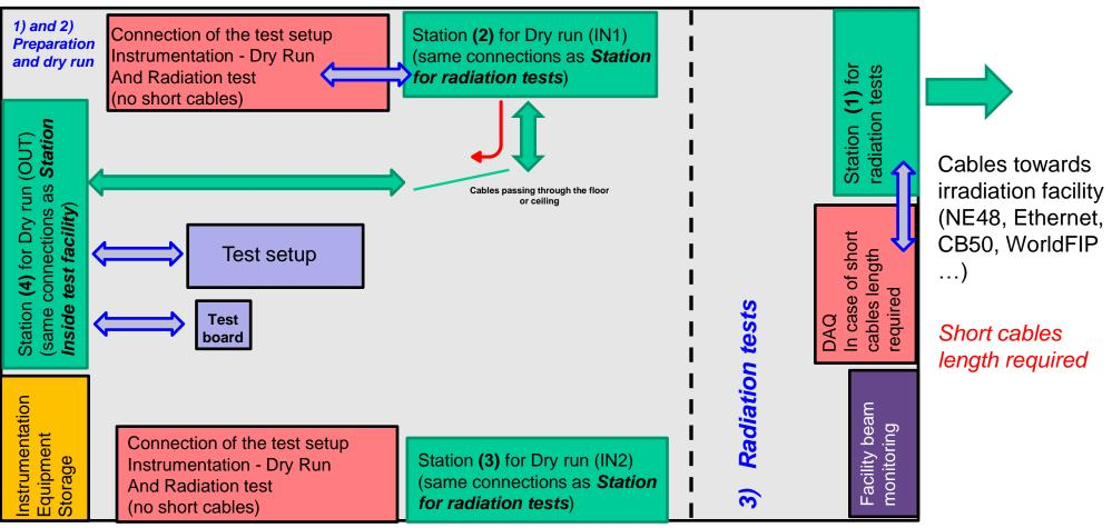
Cables length from Station (2 or 3) to Station 4 = Cables length from Station (2 or 3) to irradiation facility
