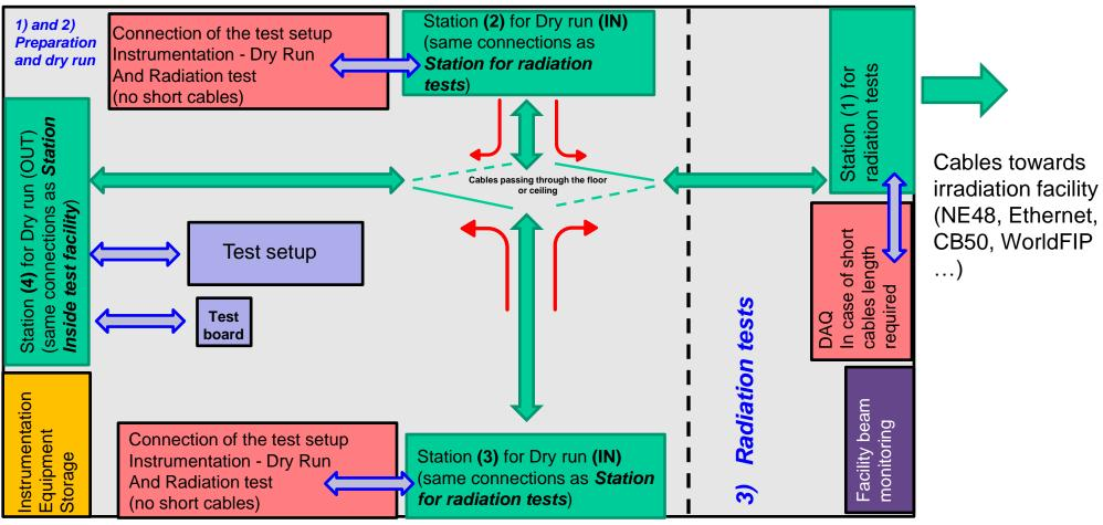
Cables length from Station (1 or 2) to Station 4 = Cables length from Station (1 or 2) to irradiation facility
