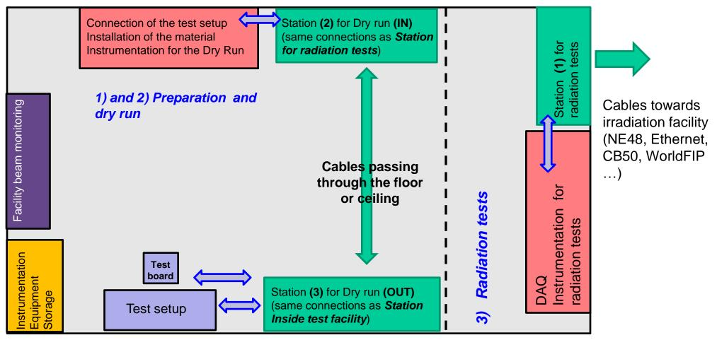
• Cables passing through the floor  $\rightarrow$  Same length than from Station (1) to the irradiation facility
