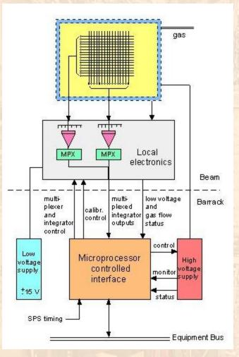
The local electronics contains integrators for each wire of the chamber and the integrated charge is multiplexed and send to the acquisition system on the surface, often through several hundred meters of cable.
