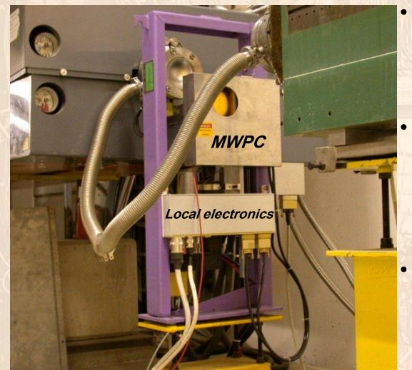
MWPC are widely used in the experimental areas for profile measurement.
