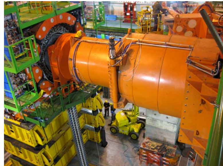
HF tested at beam height with rotational shielding closed, Sept. 2007
