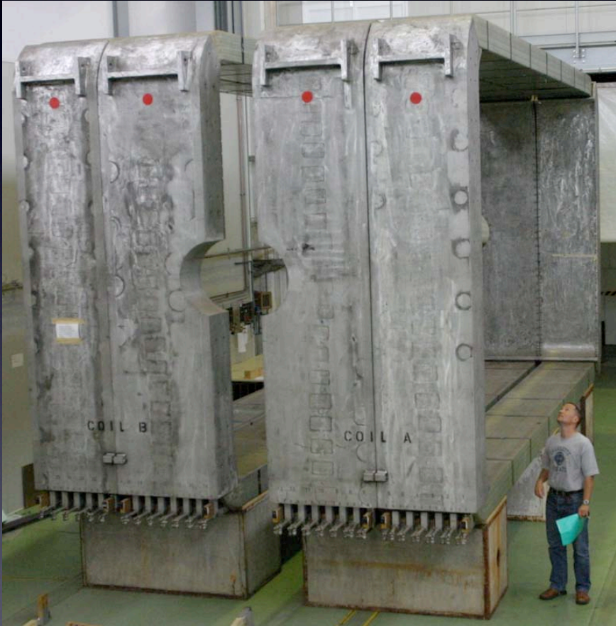
Tested to 25 bars, up to 1.35 kV for 30s
