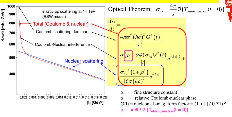
Measurement of  $\rho$  by studying the Coulomb – Nuclear interference region down to  $|\mathbf{t}| \sim 6 \times 10^{-4} \, \text{GeV}^2$
