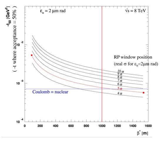
The pots have to approach the beam to a distance  $\sim 4~\sigma$  Beam emittance  $\epsilon_n < 2~\mu m$  rad
