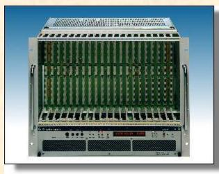
21 slot 9U crate (with 6U section) for 19" racks
