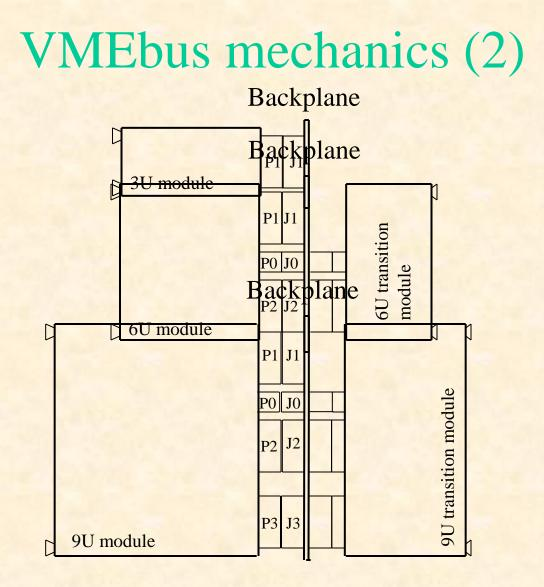
In 6U and 9U systems there can be transition modules installed on the rear side of the backplane. Transition modules do not connect to VMEbus but just to the module on the opposite side of the backplane via the user defined pins of the J0, J2 and J3 connectors
