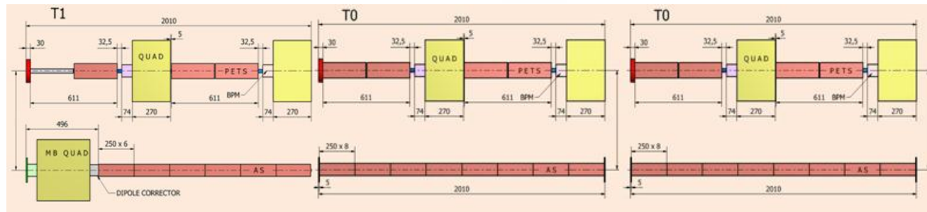
Schematic layout of CLIC Modules in CLEX
