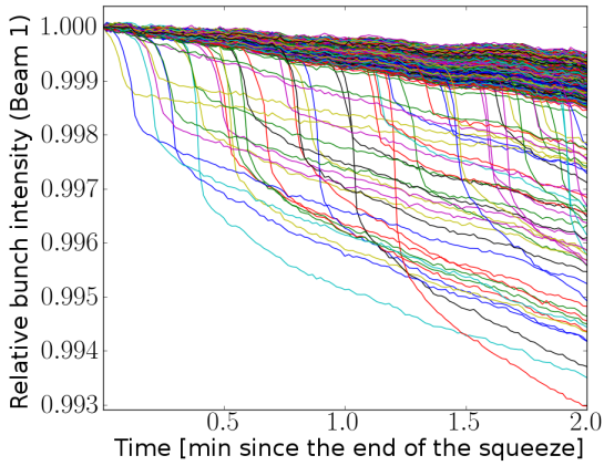
Figure 1: Bunch by bunch losses in beam 1 during an end of squeeze instability as a function of time for Fill 2648 with negative octupole polarity (top picture) and Fill 3250 with positive polarity (bottom plot).
