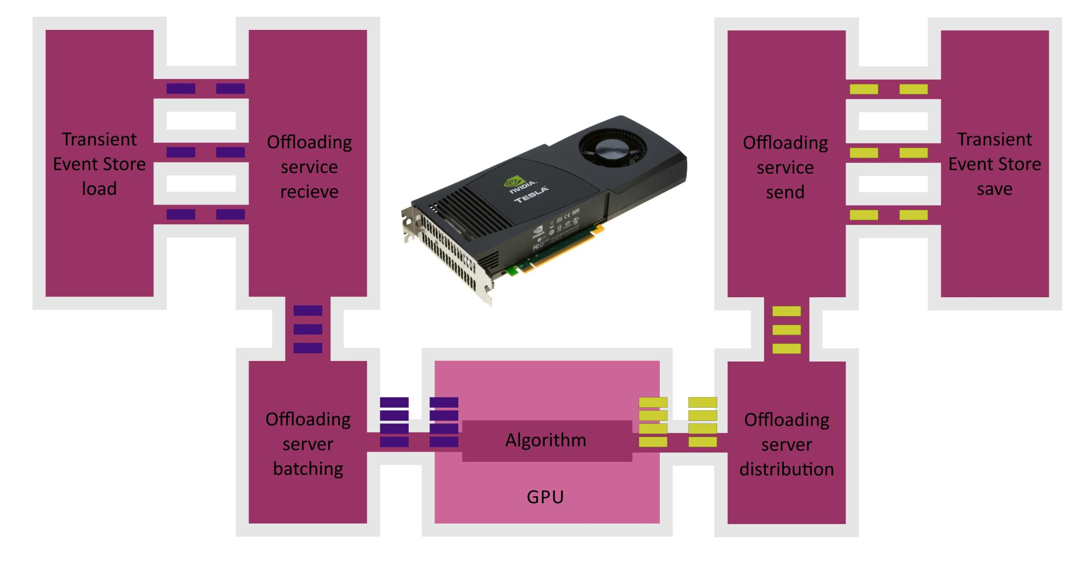
TES is converted to a coprocessorfriendly SoA format and back. The converted data is sent to the GPU kernel.
