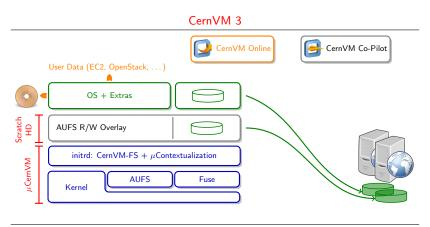
Twofold system:  $\mu$ CernVM boot loader + OS delivered by CernVM-FS
