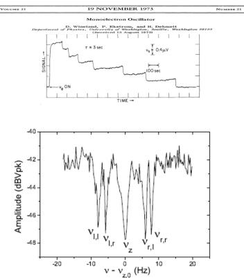
Five simultaneous signals by one single trapped particle
