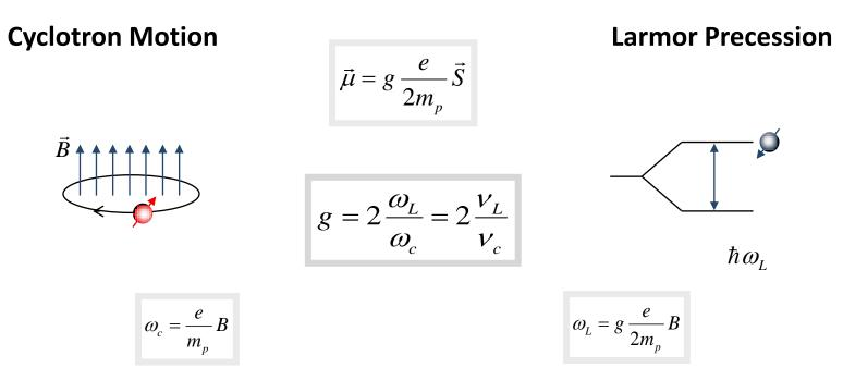
Determination of the g-factor reduces to the determination of a frequency ratio -> in principle a very simple experiment
