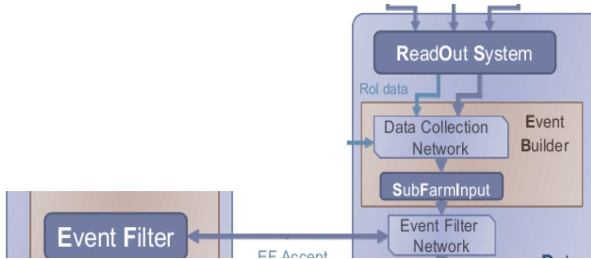
→ Pull protocol using TCP over Ethernet
