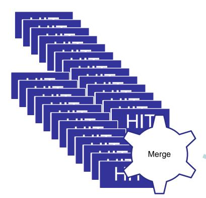
Merge 50 HITs files into one JumboHITS file JumboHITS file order 5 GByte and contains 2500 events Simulation and merging run at the Tier-2's JumboHITS file uploaded to Tier-1 Reconstruction runs in Tier-1's
