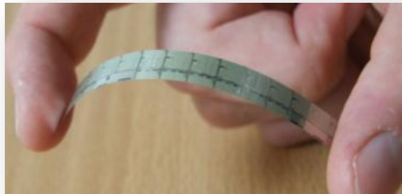
Sample of IPD of 250nF/mm 2 thinned at 60μm
