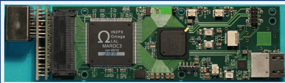
Adjustable gains in front-end MAROC3 or CLARO
