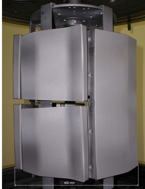
W-coated CFC tiles by CMSII technology for JET divertor
