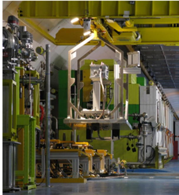
Figure 1: Remotely controlled installation of an experiment on the target position. A standardized cage (metal bottom with frame) hosting the experiment (central aluminum box on foot) is moved using the overhead crane. The final position is determined by the black pins on the fixed installation. Automatic connections for electrical lines and cooling circuits allow a fully remotely guided installation and removal of the experiment, an important feature in such environments with radio-active material.
