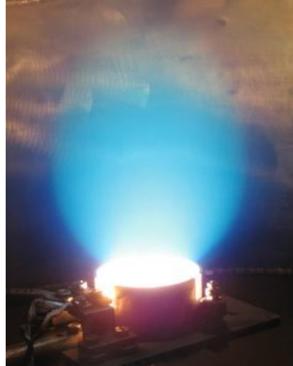
TVA plasma running in pure chromium vapors
