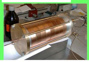
The vertical modes have been measured before the final assembling of the structure and the sampled dispersion curve has been obtained.
