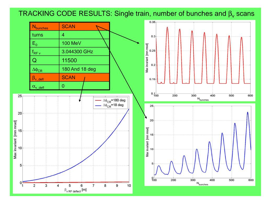
The *profile of the vertical oscillation* as a function of the bunch positions is the *same shot by shot*
