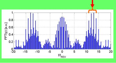
The *profile of the vertical oscillation* as a function of the bunch positions is the *same shot by shot*
