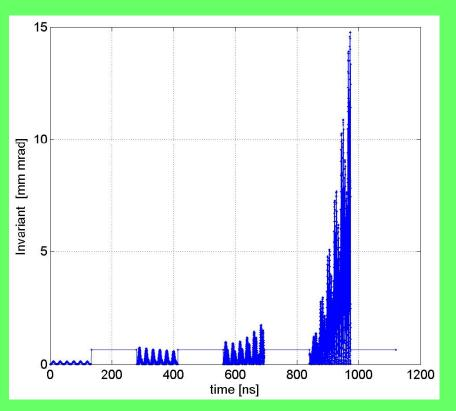
The *profile of the vertical oscillation* as a function of the bunch positions is the *same shot by shot*
