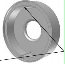
Metallic rods have been inserted to split in frequency the deflecting mode with vertical polarity.
