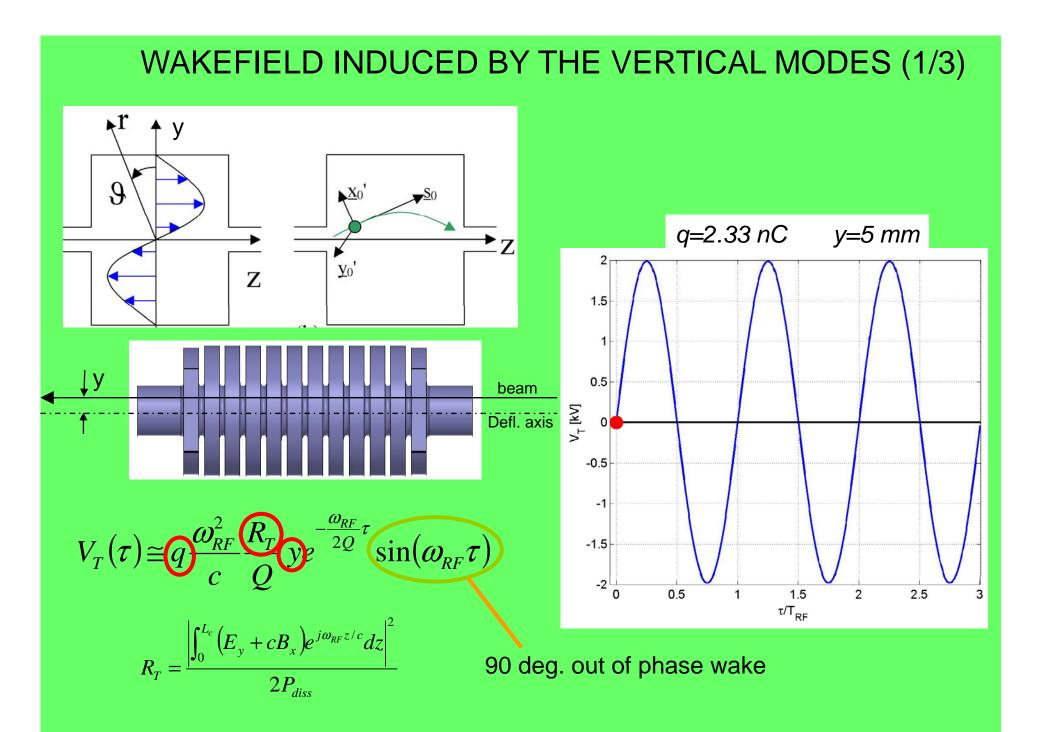
The *profile of the vertical oscillation* as a function of the bunch positions is the *same shot by shot*
