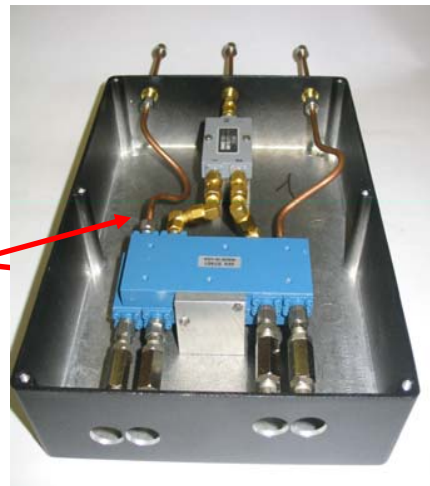
Signal processing electronics of the re-entrant BPM
