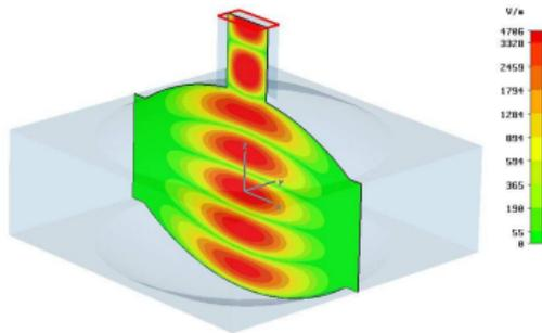
Electromagnetic field in the NCR cavity at 12 GHz for the  $m = n = 0$  and  $q = 4$  mode.
