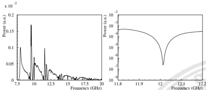
Minimum at 12 GHz: small transit time factor for the mode with  $m = n = 0$  and  $q = 4$ , which has  $E_z(s) \propto e^{-s^2/2w_0^2}$ :
