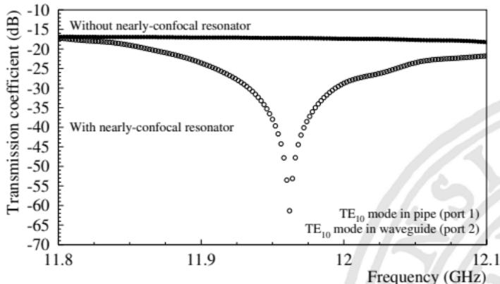
CST simulations show a clear rejection of the  $TE_{10}$  mode of the pipe around the resonant frequency of the NCR.
