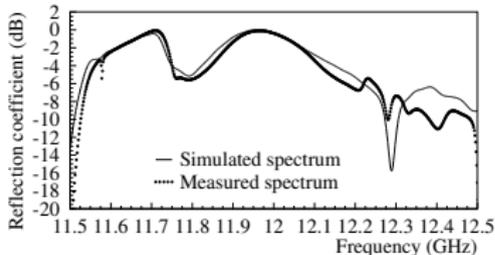
A clear rejection of incoming modes at the NCR resonant frequency.
