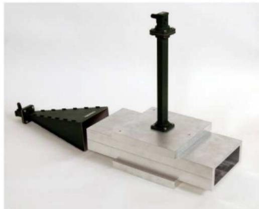
The horn antenna allows to inject TE and TM modes into the rectangular pipe.
