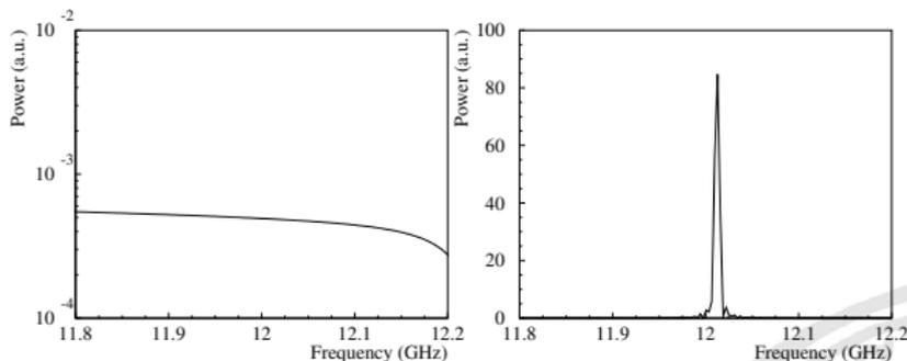
For a bandwidth larger than 50 MHz, the output power during the passage of a bunch train is 500 W.
