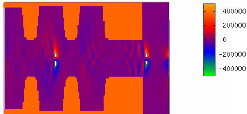
Transverse Electric Field E_x (V/m) in the RF Gun at 0.5 nC
