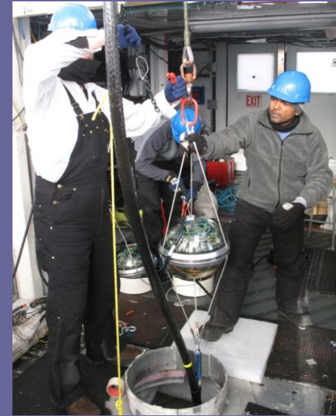
Installing an IceCube string
