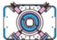
TEVATRON B = 4.5 T Bore : 76 mm
