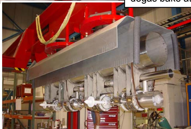
3.9GHz Cryomodule Mockup Assembly
