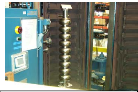
1.3GHz bare cavity hydrogen degas bake at CAF-IB4
