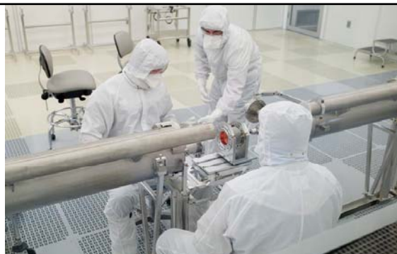
Cryomodule #1 (CM1) string assembly in the cleanroom
