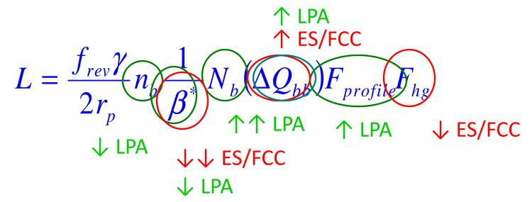
where  $(\Delta Q_{bb})$  = total beam-beam tune shift;
