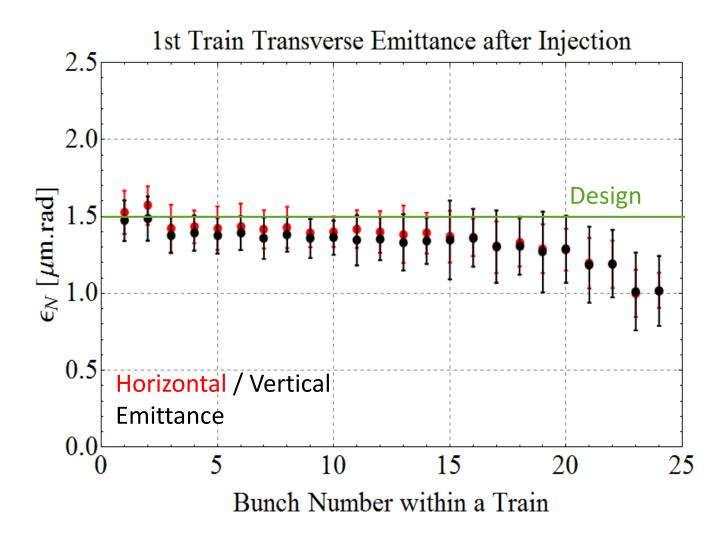
Wire Scanner data of the first train in Pb-p Mode 2013 (Pb in Beam1)
