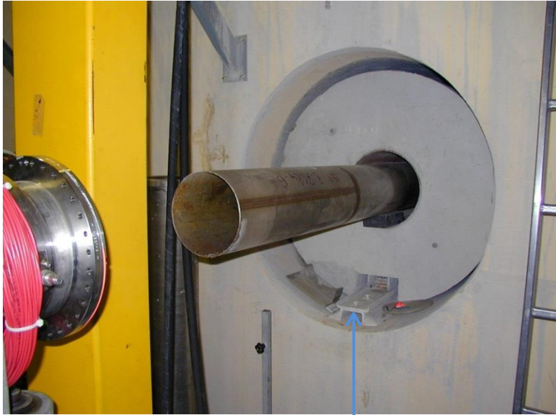
Rail's surface where the concrete blocks roll d = 807 \text{ mm}
