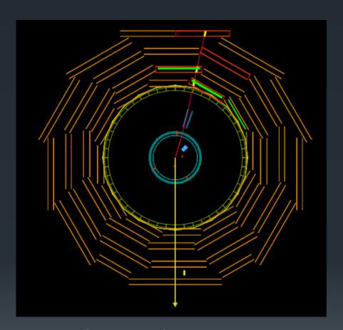
Muon (red track) traversing whole detector, leaving hits in outer layers. Missing energy represented by yellow arrow
