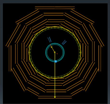
Electron (yellow track) stopping in the ECAL. Missing energy represented by yellow arrow
