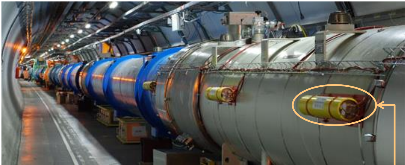
An ionization chamber, a specific type of Beam Loss Monitor in the LHC Ring.
