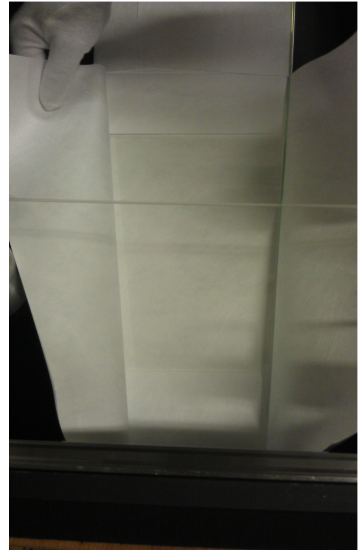
Tyvek paper covering the scintillator tile
