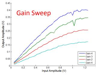
•The AOH boards consist of 4 selectable Gains: 0,1,2 and 3.
