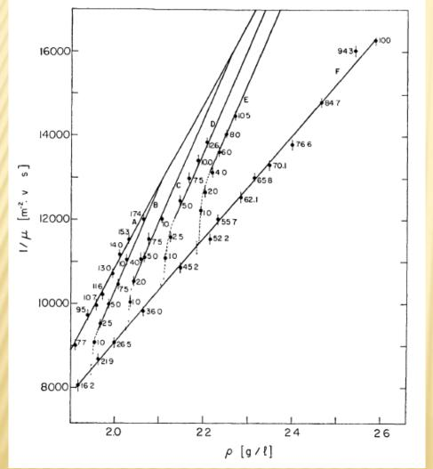
Curve A : argonmethylal Curve B : argon 80 %-isobutane-methylal Curve C :argon 70 %-isobutane-methylal Curve D : argon 60 %-isobutanemethylal Curve E : argon 50 %-isobutane-methylal
