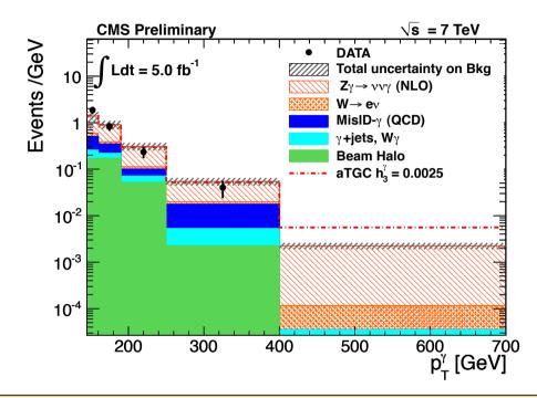
$$\sigma \text{ (pp} \to Z\gamma + X \to vv\gamma + X, \\ E_{T}^{\gamma} > 145 \text{ GeV, } |\eta^{\gamma}| < 1.4) @ \text{ TeV:} \\ 21.3 \pm 4.2 \text{ (stat.)} \pm 4.3 \text{ (syst.)} \pm 0.5 \text{ (lumi.) fb} \\ \text{NLO prediction (Baur): } 21.9 \pm 1.1 \text{ fb} \\$$
