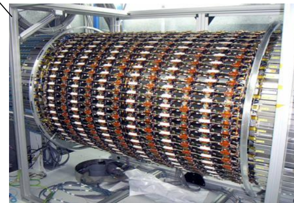
6000 sensors and 980 modules of barrel SCT system, KEK, Tsukuba, Okayama, Hiroshima ...
