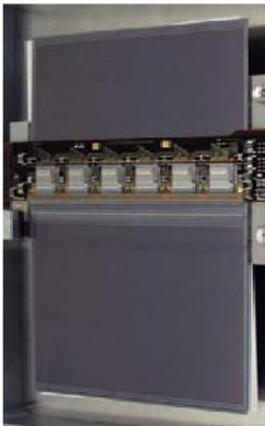
A cylindrical SCT barrel structure, radius 299 mm, length 1492 mm, tiled with rectangular modules constructed using silicon sensors supplied by Hamamatsu Photonics
