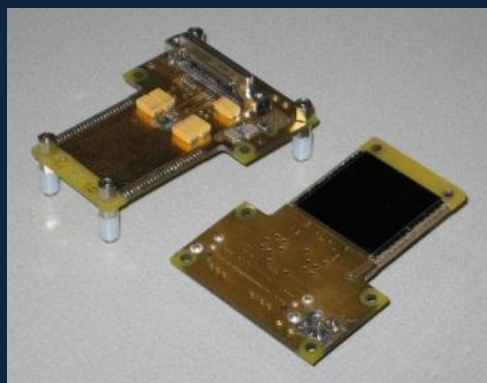
Medipix2 Quad Pixels: 512 x 512 Pixel size: 55 x 55 \mu\text{m}^2 Area: 3 x 3 \text{cm}^2
