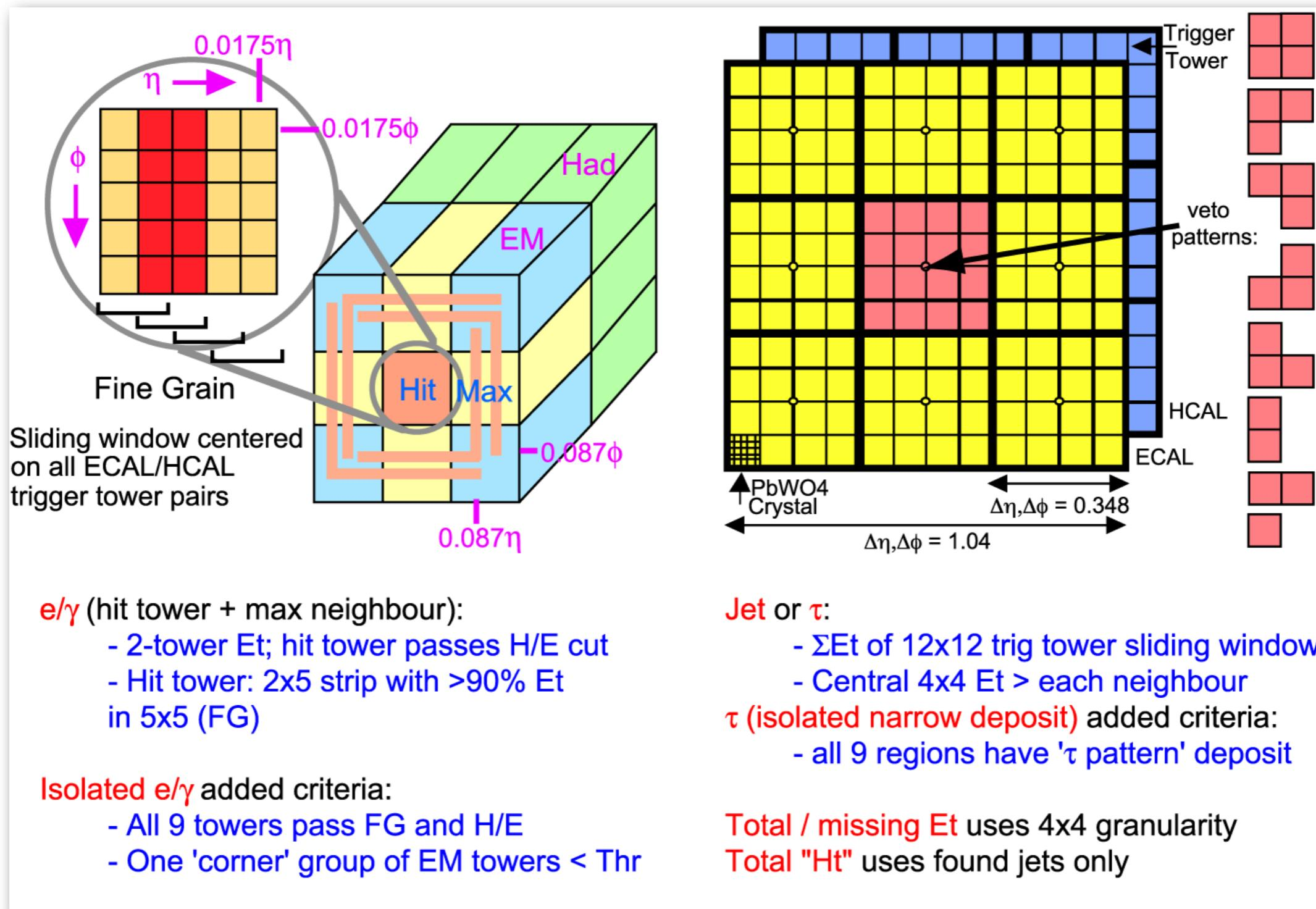
► e.g. CMS calorimeter trigger – electron / photon ID
