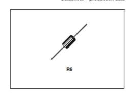
Type 2: **BZW50-180B**: Transil™, Transient voltage surge suppressor (TVS), bidirectional
