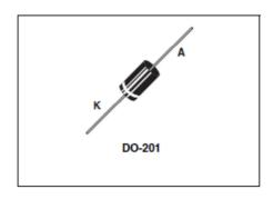
Type 1: **1.5KE-220CA**: Transil™, Suppressor diode; bidirectional
