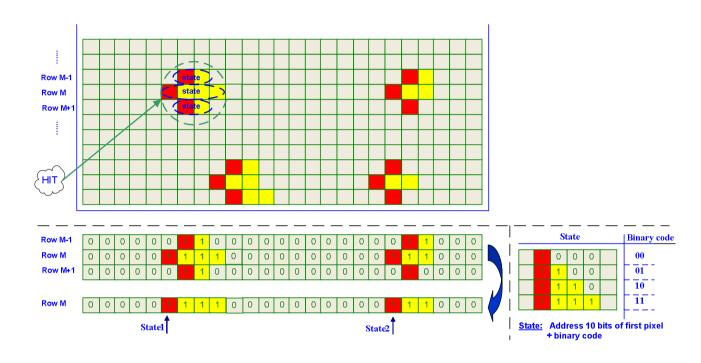
Encoding of adjacent hit pixels in a row (up to four in one group) plus a common row address (if more than one state/row), means data compression but no real clustering.
