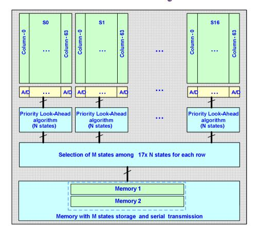
M22+ array size: 1088 x 544 pixels, 18.4 µm pitch (exactly as M22)
