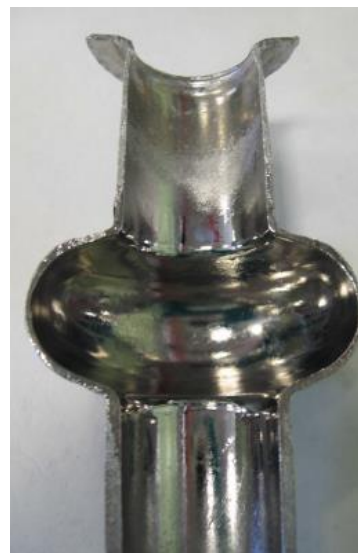
6GHz half-cavity after treatment in horizontal position
