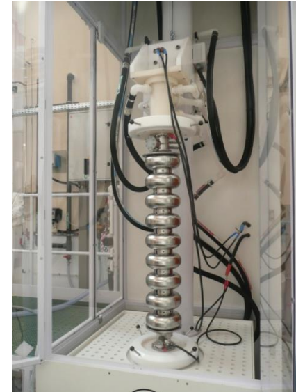
Fermilab TB9RI025 cavity Prior to VEP
