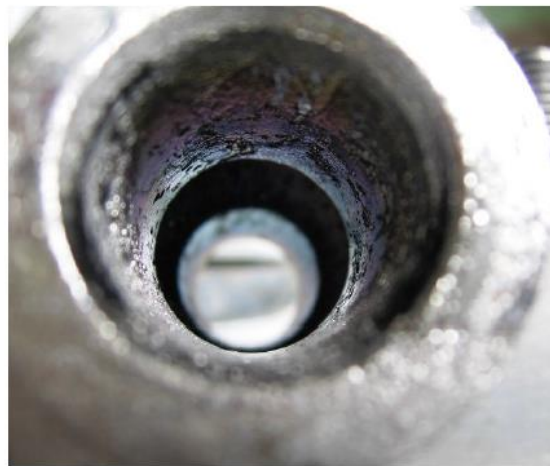
6GHz cavity after treatment in vertical position
