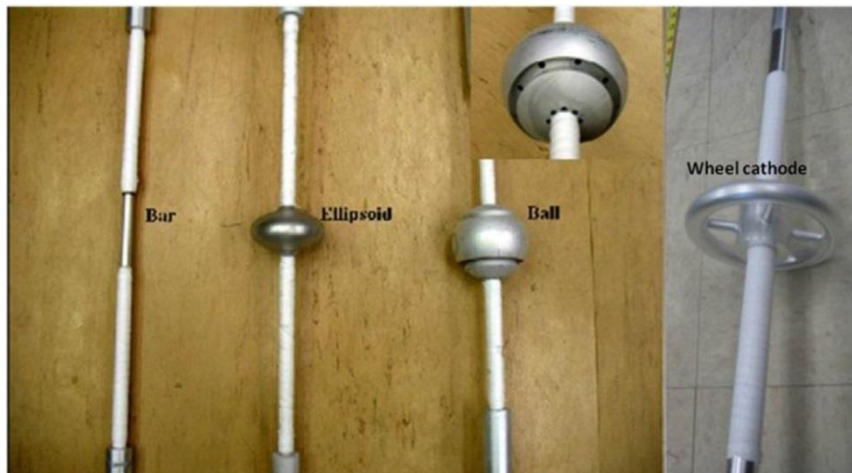
Cathodes tested at J-Lab during BEP studies
