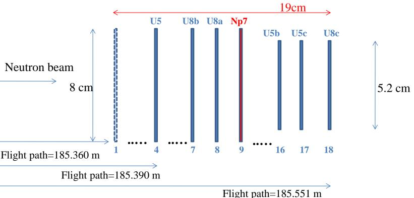
•Each detector signal was recorded at a FADC channel every 25 ns in a time window of 100 $\mu$ s. •Reference for cs calculation:  $\sigma(U235(n,f))$  up to E=2 MeV and  $\sigma(U238(n,f))$  above.
