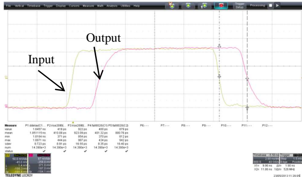
Fig. 21a: LVDS Receiver, propagation delay
