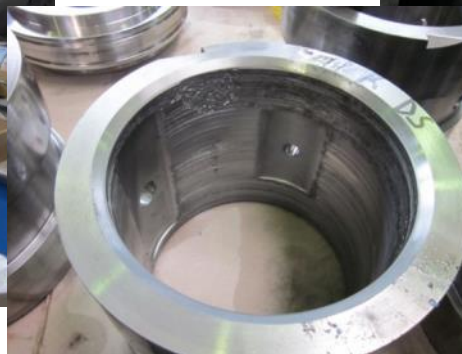
Damaged slide bearing seat (QSCB-4-CP1)
