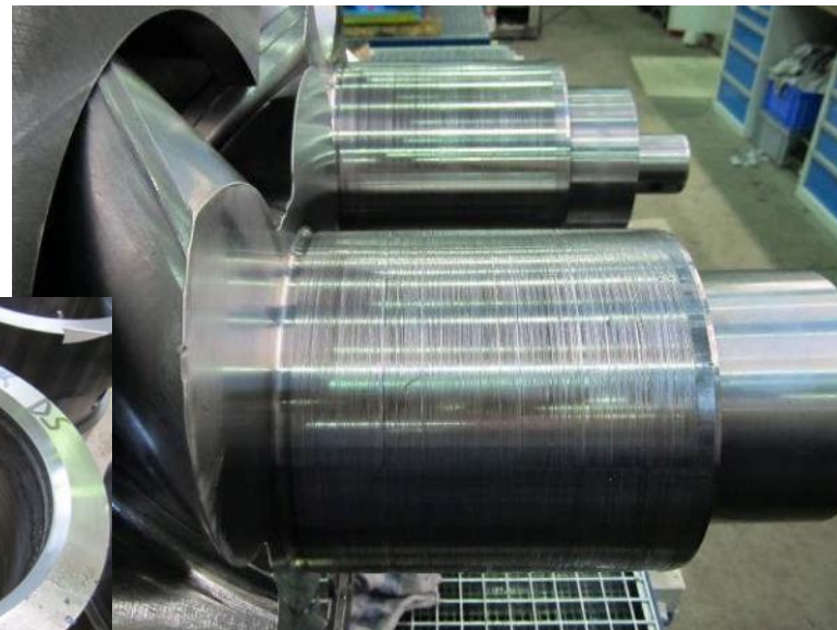
Damaged slide bearing seat (QSCB-4-CP1)
