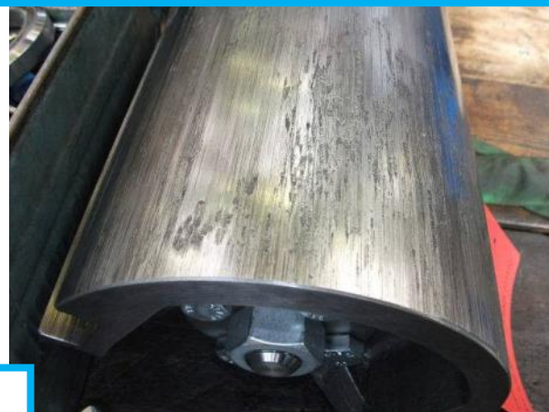
Damaged slide bearing seat (QSCB-4-CP1)
