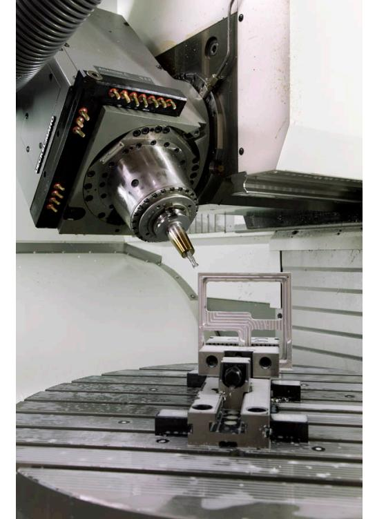
Here automatic 5 axis machining
