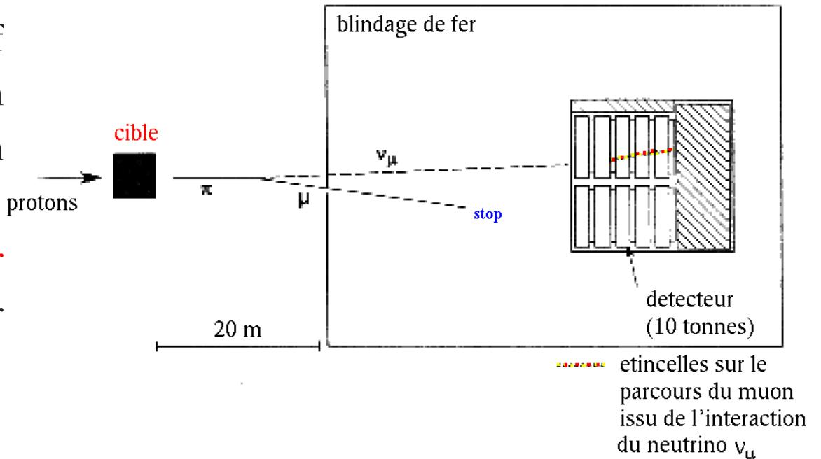
Schwartz, Lederman, Steinberger and Gaillard built a spark chamber (a 10 tons of neon gas) to detect  $\nu_\mu$
