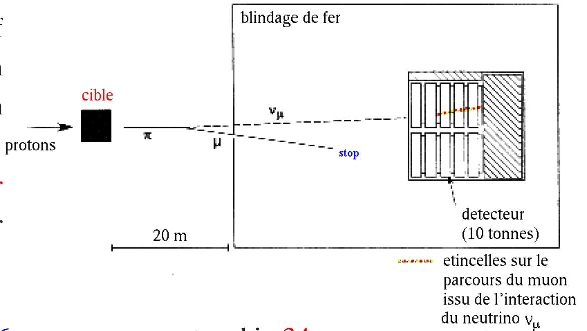
Schwartz, Lederman, Steinberger and Gaillard built a spark chamber (a 10 tons of neon gas) to detect  $\nu_\mu$
